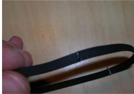
Reconnect the belt using the glue, don't exaggerate: a small quantity is enough. Spread the glue on the belt's cut using one needle. Important: Try to be sharp when joining together the two belt's part; it's fundamental in the correct belt's spinning .
