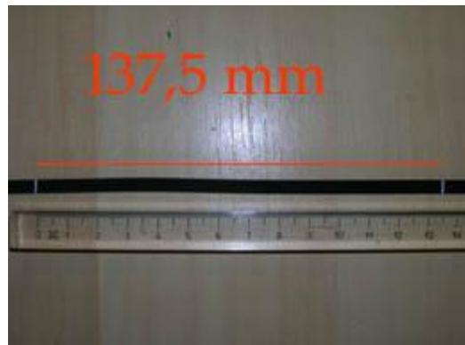
Always keeping the belt taped on the surface, take two marks with a marker at a distance of 137,5mm one to each other. It's not important where you draw the first mark, but it's fundamental that the second is drawn at 137,5 mm from the first.
