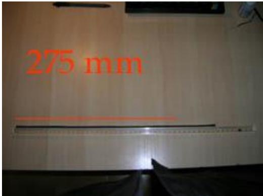
Take the new belt and make a cut with using the cutter then tape the belt on plane surface (to keep it steady) without bending it and cut it (make sharp cuts) - Do the second cut to make a belt 275 mm long.
