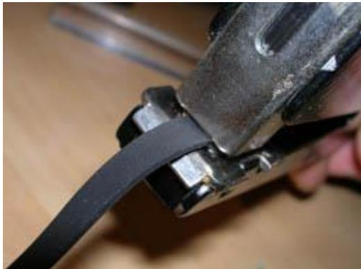
Take the stapler and use it on the belt, put two staples one on each mark made in part one. The staples must be stitched on the same way . Using the stapler don't be rude or you'll cut the belt!
