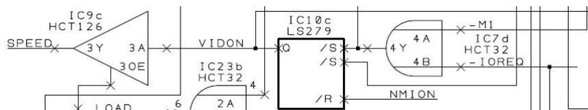
As this detection is unique there is no special use of A15 or any other address needed. Outside of video display machine code can be executed on any runtime address. The clock frequency is reduced automatically to 3.25 MHz during video mode to assure the correct display timing. The end of video display is detected by activation of NMI again.
