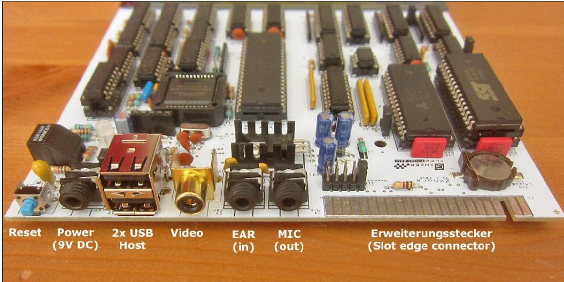
**Reset** allows reset of the current instance and return to the ZXmaster control software.
