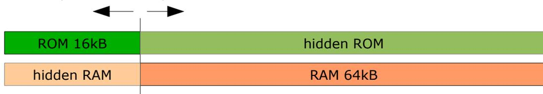
The memory layout can be defined different for any of 7 instances. It is possible to move the border on request to access some hidden memory areas to place additional drivers in ROM area which use only sparse RAM and can release RAM areas after use. On the other hand it is possible to use additional RAM for storing temporary data when hide ROM areas.
