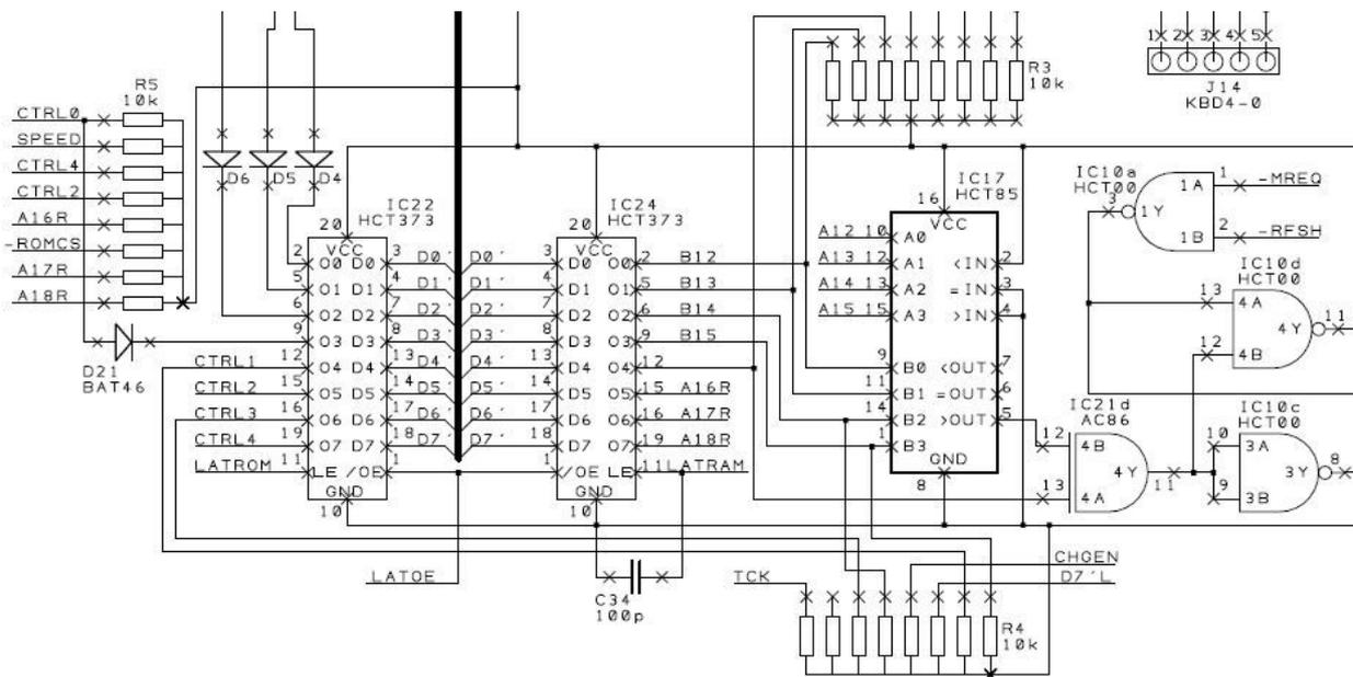
The schematic shows the latch control. The RAM latch controls an address comparator which compares the programmed address with the current address and activate RAMCS when the current address is greater than the programmed and otherwise activates ROMCS. Bit 4 allows to swap ROM and RAM.
